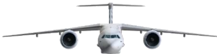
Figure 85 – Evolution of SMR+ concept as a high-wing configuration with VPF engines.
