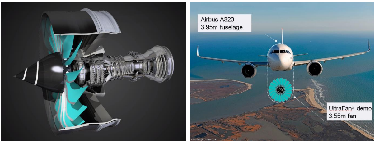
Figure 14 – Rolls-Royce Ultrafan® engine concept (left), and comparison of fan diameter with A320 fuselage diameter (right), courtesy Rolls-Royce & Airbus.
