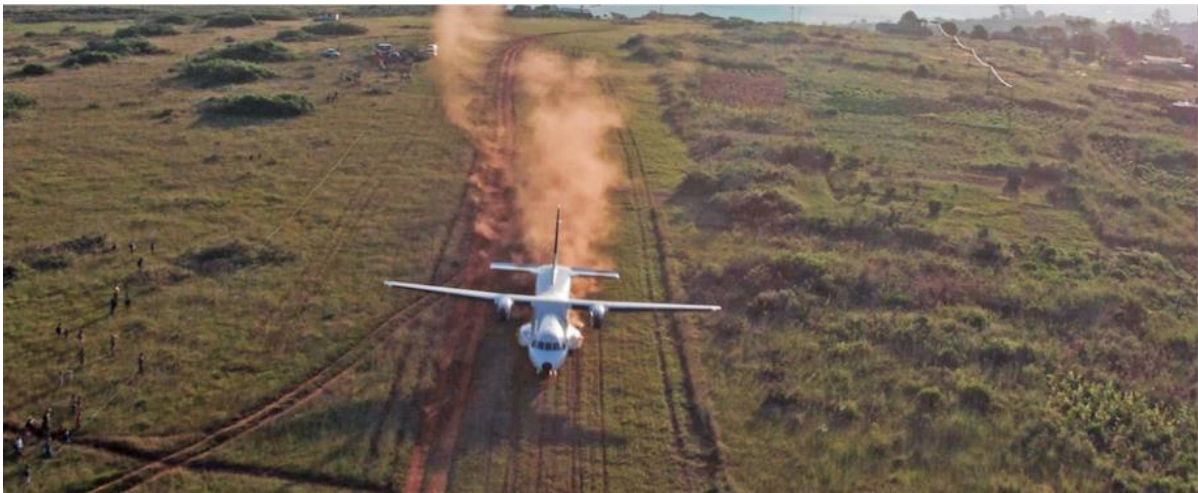
Figure 31 – C-295 landing on a grass strip in Kenya, courtesy Airbus Defense & Space.
