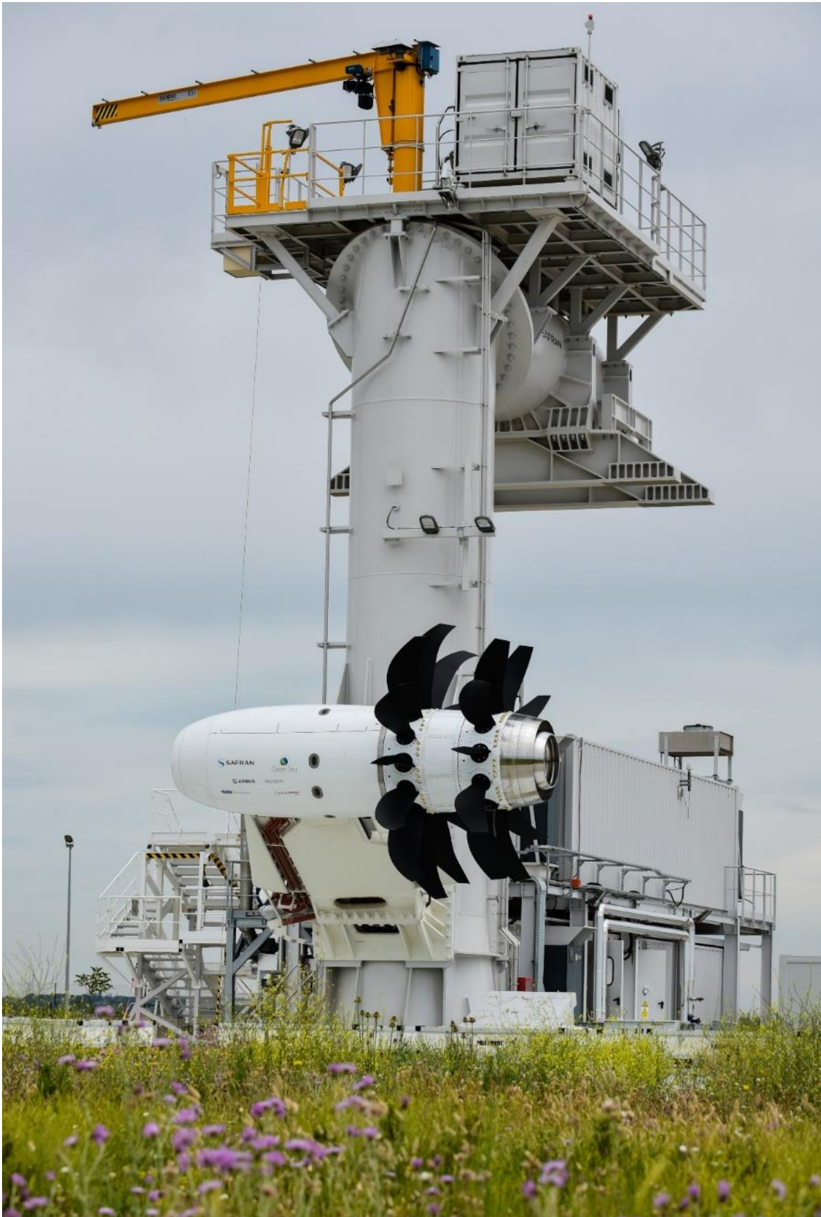
Figure 24 – CROR ground test demonstrator at Safran Aero Engines' ground testing facility for Open Rotors and Ultra High By-Pass Ratio engines (Istres, France) – Courtesy SAFRAN.
