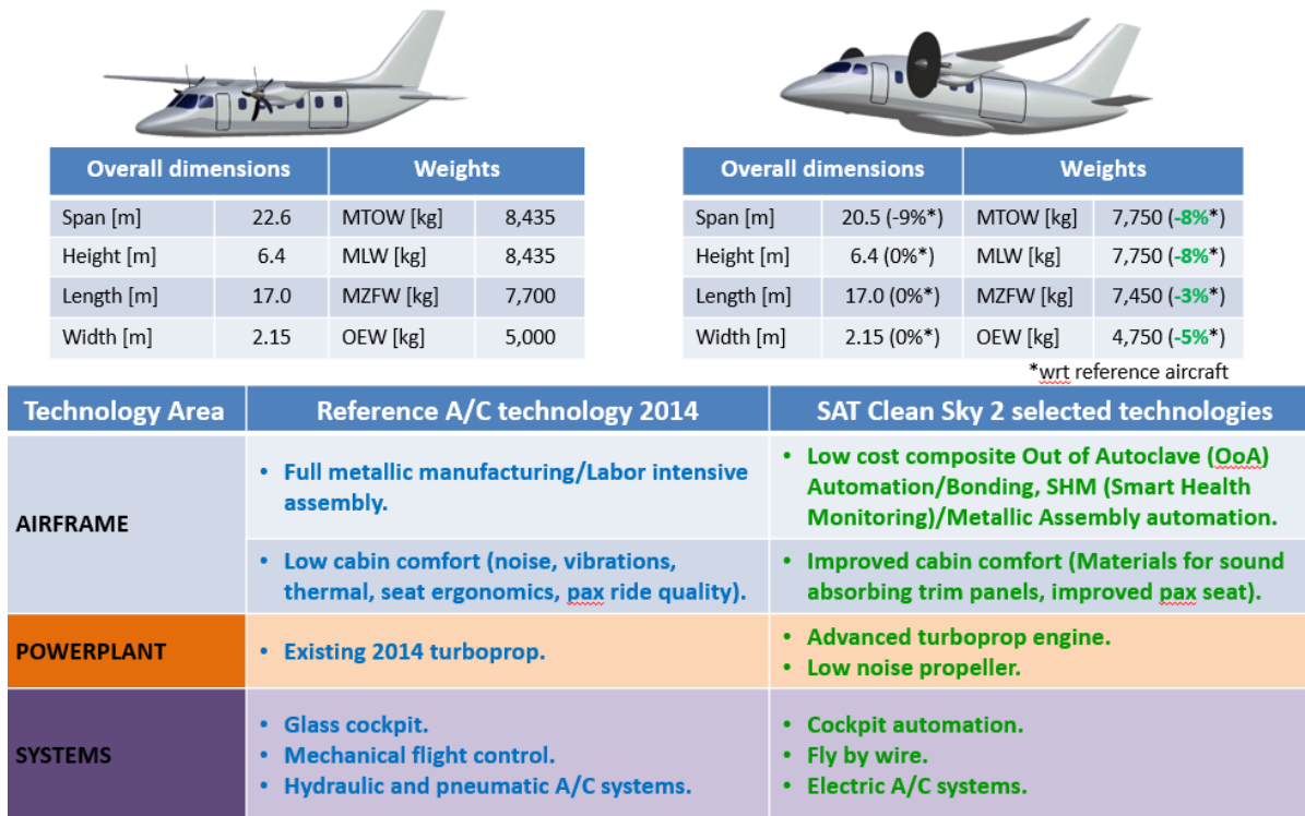
Figure 36 – Comparison of overall dimensions and weight of 19 pax reference and concept aircraft.
