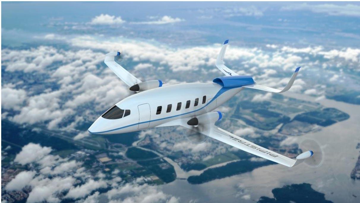
Figure 45 - Artistic impression of a 19-seater with liquid hydrogen hybrid propulsion technology (based on preliminary sizing evaluation), courtesy Pipistrel, https://www.pipistrel-aircraft.com/unifier19-2 .
