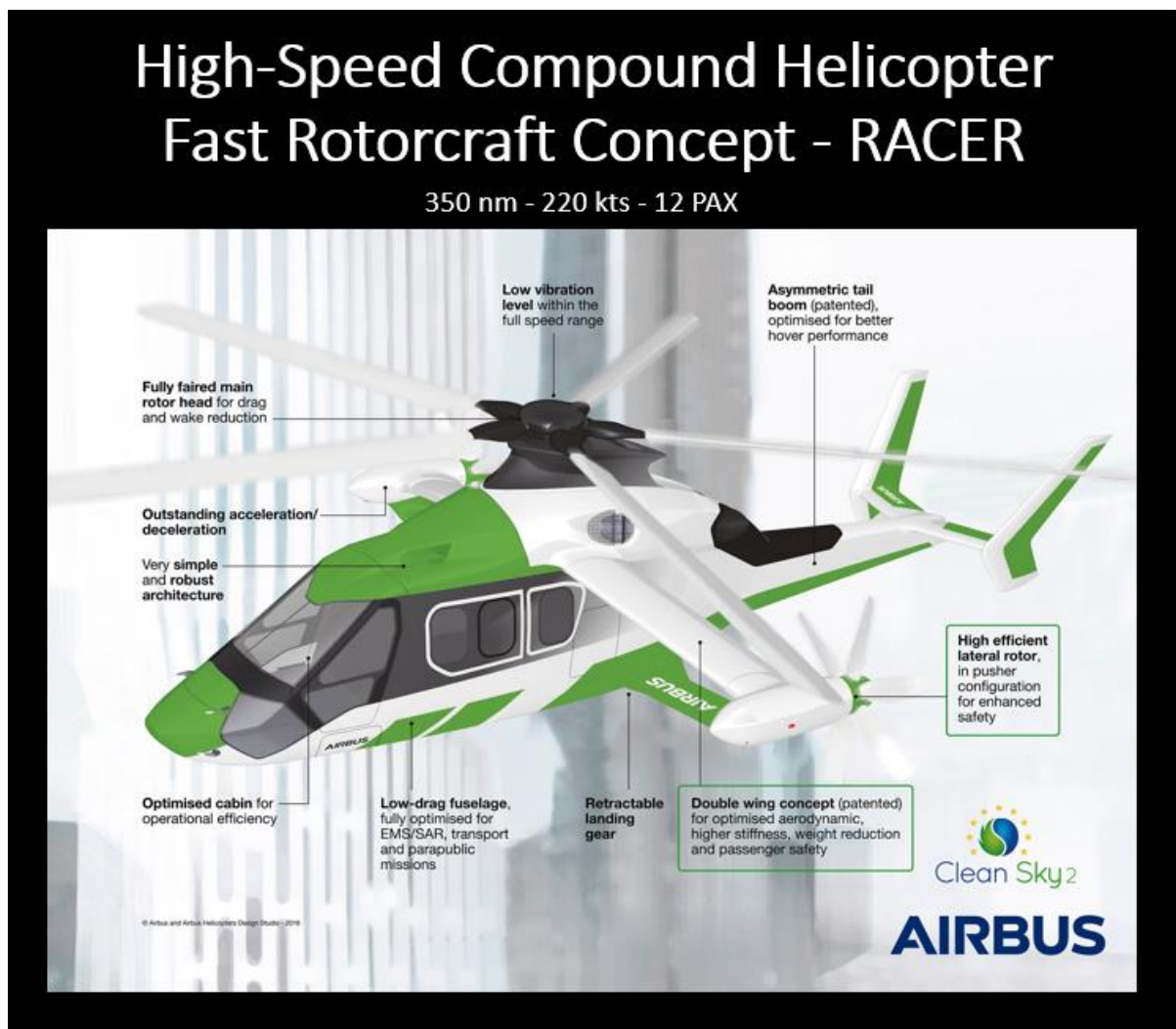
Figure 51 – The Airbus RACER Concept and its main technology features.
